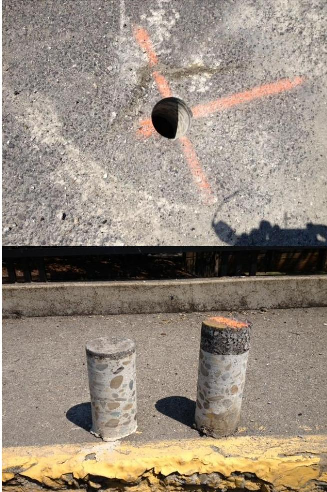
Coring of the deck revealed solid, continuous cores. The visual inspection of the cores provided additional assurance on the structural integrity of the bridge. Strength testing of the cores will be performed to complete the evaluation.
